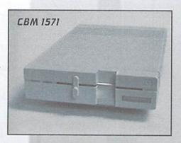
additional capabilities to the 1571. It could read from and write to most disk formats from other CP/M machines. It could even use an MS-DOS formatted disk that was intended for those double-sided IBM drives.
